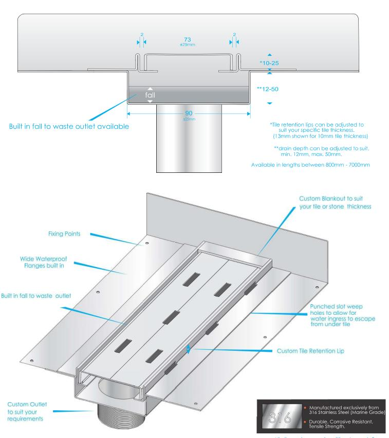
All dimensions are in millimetres, +/- 3. Drains 1.2mm Stainless Steel
