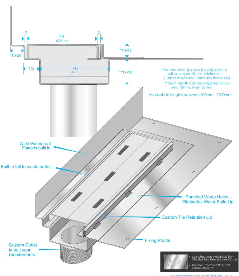
All dimensions are in millimetres, +/- 3. Drains 1.2mm Stainless Steel
