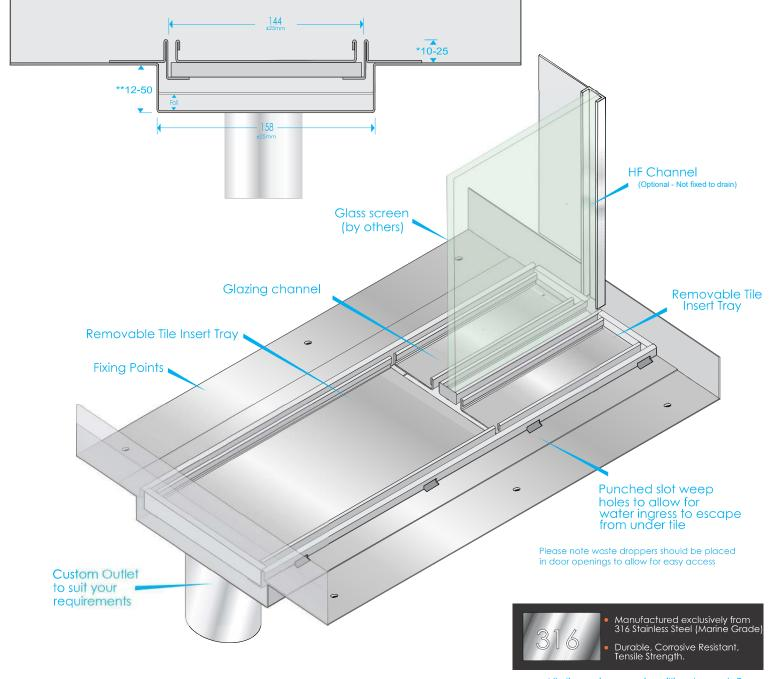
All dimensions are in millimetres, +/- 3. Drains 1.2mm Stainless Steel
